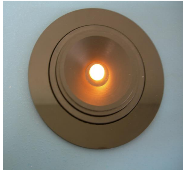
Figure 1. The reading tip of the colorimeter device used as a guide for determining the shape and diameter of the porcelain discs.
