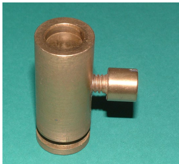
Figure 1. Stainless steel mold for the standardized veneering purposes.
